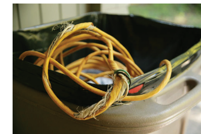
Throw away frayed extension cords
