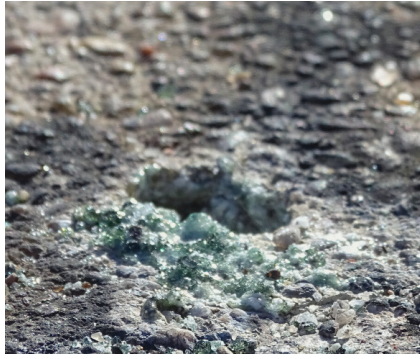
The downed power line was powerful enough to create glass from concrete and create holes and divots in the concrete under the bubbles.
