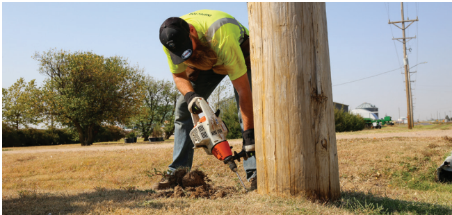
The majority of decay occurs in the first 18 inches below the ground. Inspectors bore into the pole at an angle to locate any pockets of decay below the ground.
